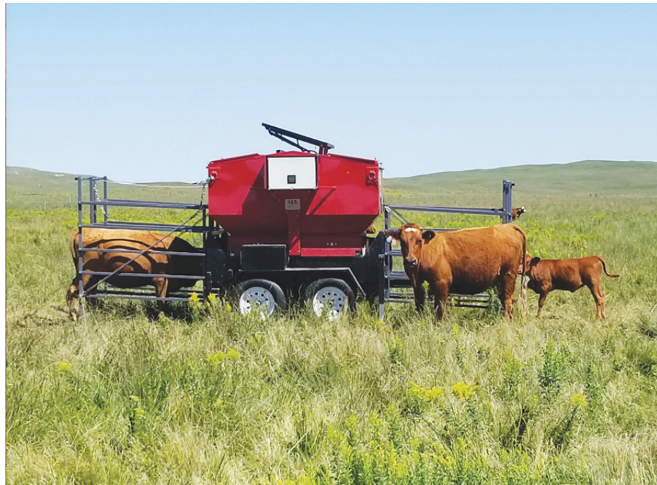
Technology in the Smart Feeder allows monitoring and control of individual livestock feed diets and intake. Courtesy photo
