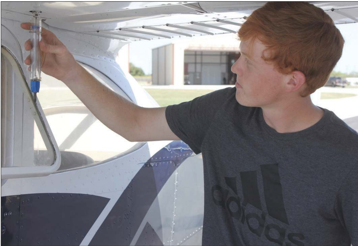
Ryan Majors checks the wing tank for condensate during aircraft pre-flight inspection. Majors is the recipient of a grant from Experimental Aircraft Association Chapter 1008, based in Gillespie County. Funding is provided by the Ray Foundation, Inc. — Photo by Lindy Segall
