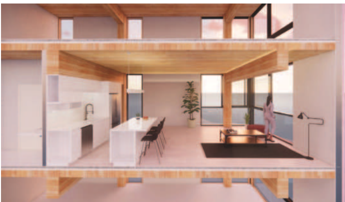
A section of Return to Form, detailing how the post and beam mass timber structure comes together.
