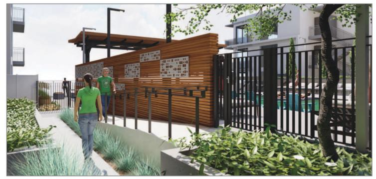
Often a portion of the amenity deck must be elevated to accommodate the pool, resulting in added stairs and ramps to provide Americans with Disabilities Act-compliant egress. One of the design challenges in this scenario is integrating stairs and ramps into the overall design while providing required pool fencing and associated gates.
