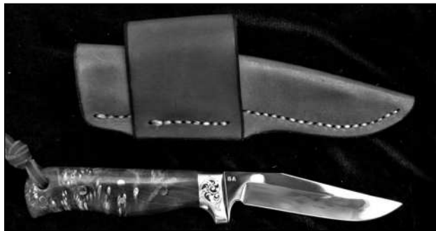
Knife, CPM 154 steel blade, brass bolster and pins, orange and black Maple burl handle, by Brian Asher. Bolsters engraved by Troy Menix. Sheath by Brian Asher.
