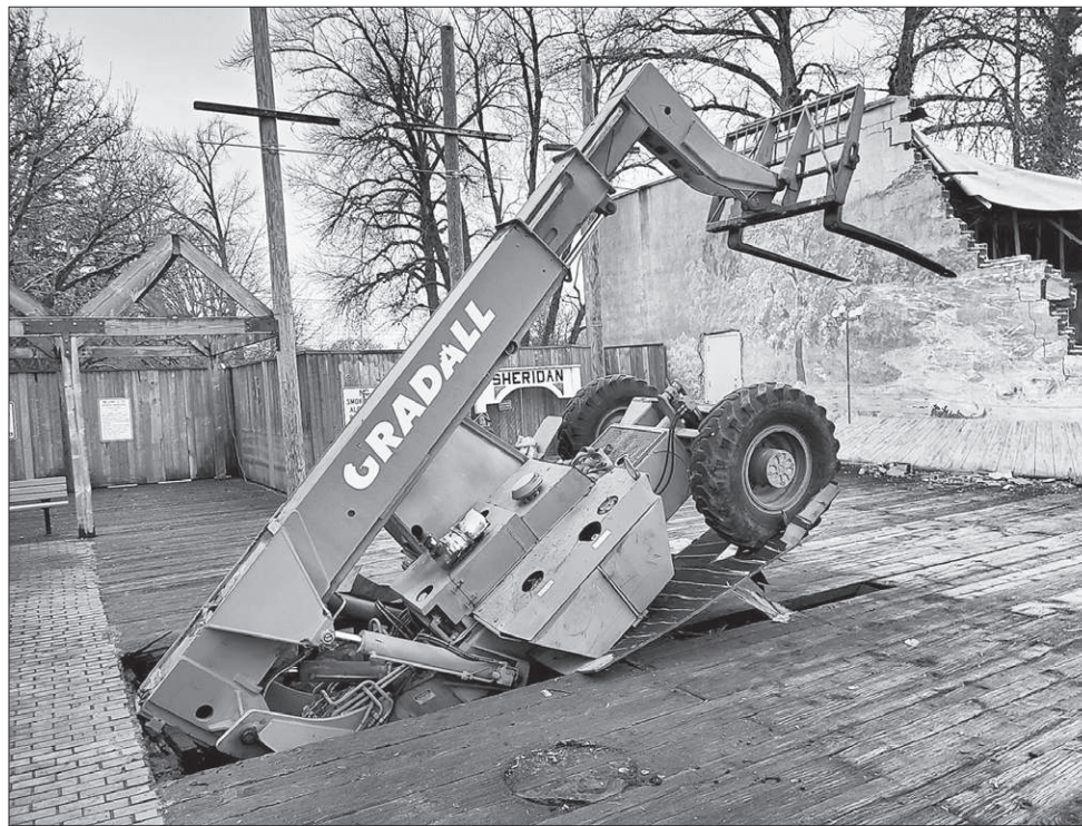
The Gradall, a piece of heavy equipment, proved too heavy for the wooden J.A. Art Hebert Memorial Plaza in Sheridan. A crane was brought in to lift the Gradall off the plaza and onto Bridge Street.
