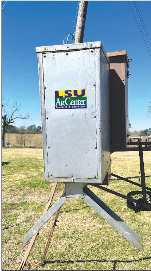
A prototype of a feral hog bait delivery system designed by LSU AgCenter scientists. The system can deliver up to 20 baits and can be activated remotely when pigs are present and actively feeding around the system.
