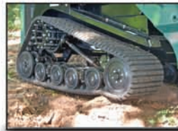
Rubber Tracks with Suspended Undercarriage
