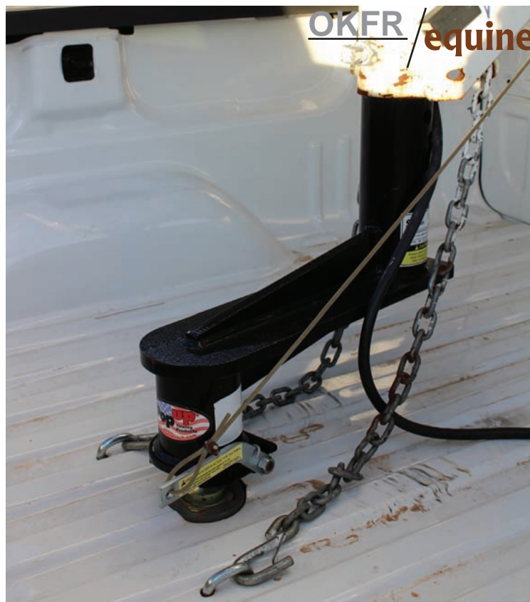
Check on the trailer hitch including ball and coupling. Keep the ball well greased. Periodically, check to see that the ball is still securely tightened and the latch on the coupling is working properly. (Photo by Jessica Crabtree)
