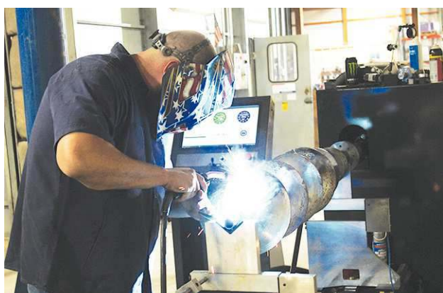
Ray Rahe, a fabricator at Abilene Machine, welds weights to an auger flighting, which balances the rotating assembly for smooth operation and longevity. Abilene Machine manufactures their own augers, which are purchased by farmers all over the U.S.
